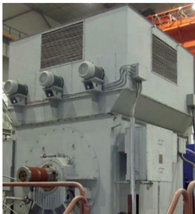
Solcon Medium Voltage Mega Soft Starter connected to an asynchronous air cooled 10kV 1627A Motor
